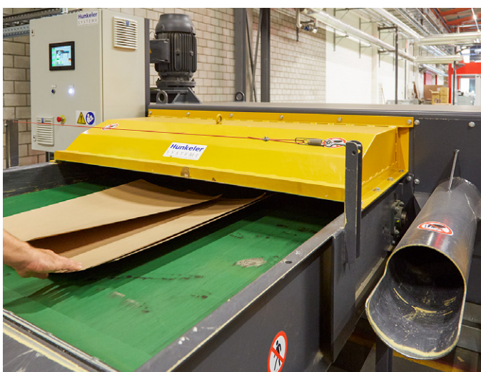
Cardboard, trimmings, and core sleeves are disposed of via a manually fed shredder.
