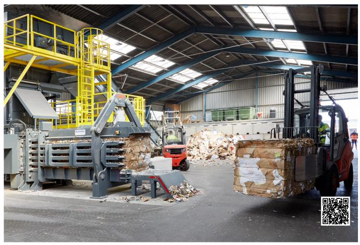
The press compresses paper and cardboard into bales weighing up to one tonne. Up to 5.5 tonnes of material are processed within twenty minutes.
