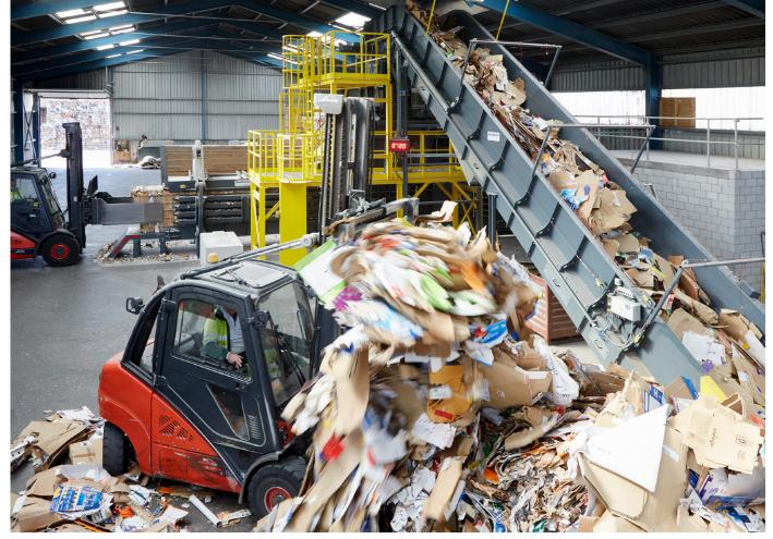
The baling press is designed for an annual volume of 15,000 tonnes. It works economically; a frequency converter controls the operation. The baler only consumes electrical energy when material needs to be compacted.
