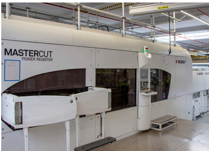
The new Bobst Mastercut 2.1 is the latest of four lines producing corrugated boxes at Smurfit Kappa MNL.
