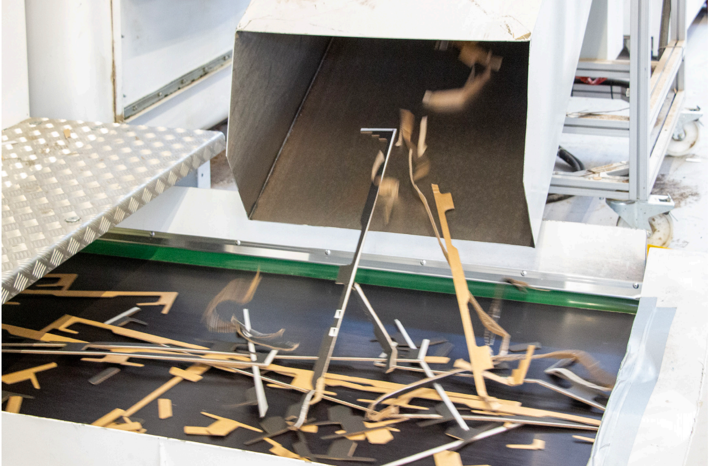
The HKZ-700 cardboard shredder shreds large, up to 150-millimetre-wide gripper edges without any problems. A conveyor belt removes the waste from the production area.
