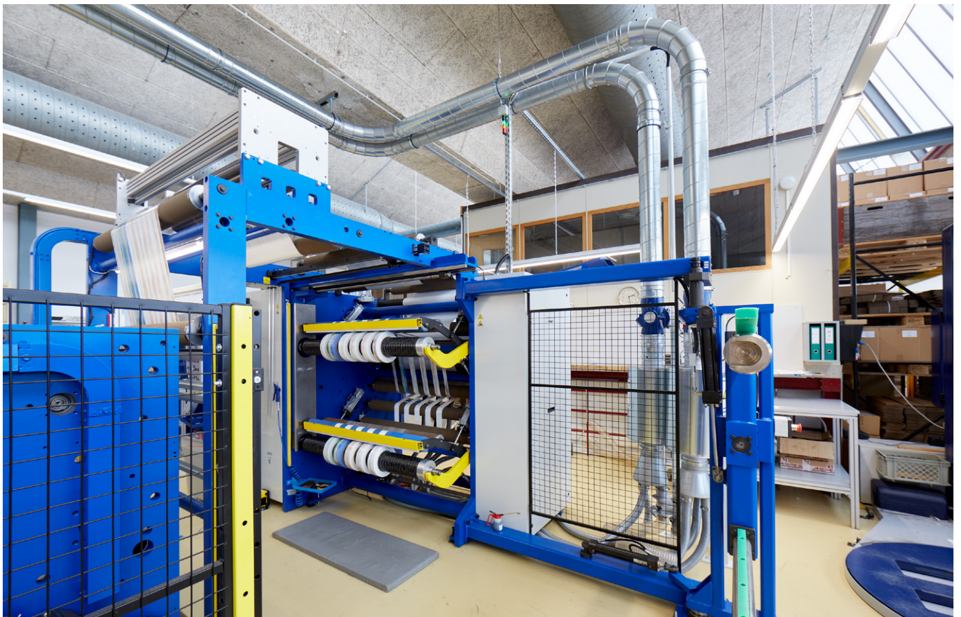
The slitter rewinder operates at a web speed of 600 metres per minute. The plastic strips are shredded in a cutter (cylindrical elements in the lower area) and disposed of via the pipelines.
