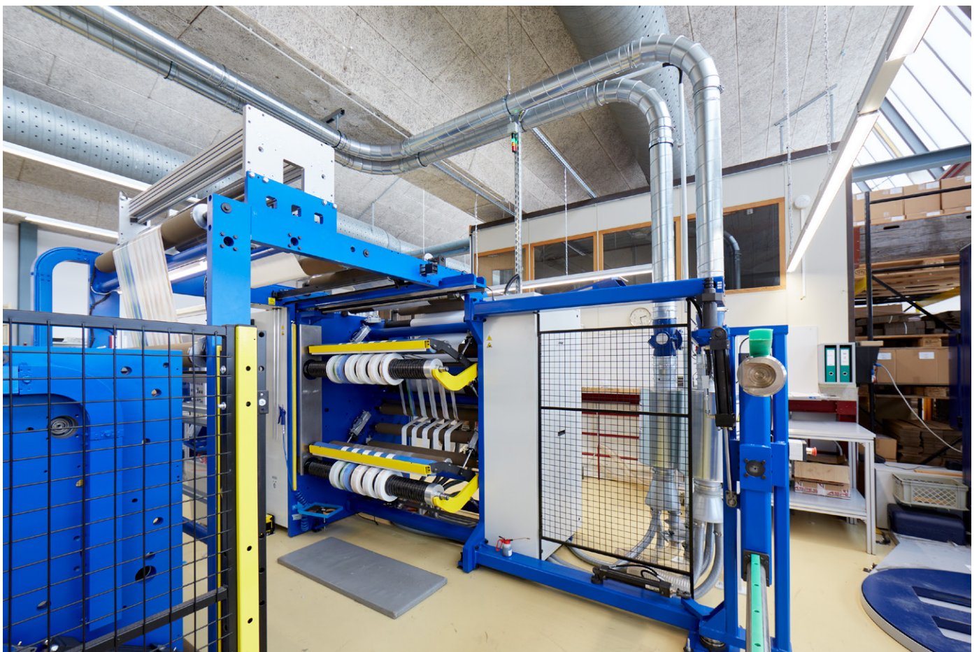
The slitter rewriter operates at a web speed of 600 metres per minute. The plastic strips are shredded in a cutter (cylindrical elements in the lower area) and disposed of via the pipelines.
