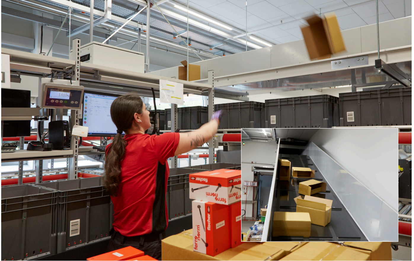
A conveyor belt (small picture) transports the emptied cardboard boxes to the outside area, where they are compacted in a press container.
