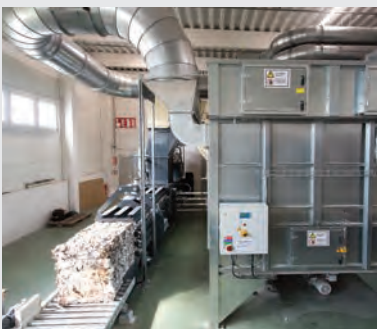
Baling press, efficient handling of die cut waste
