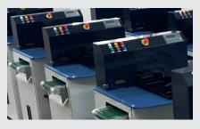
The Hunkeler Banknote-Puncher HBP 100 is a manually operated offline system for the cancellation of banknotes and other securities. A hydraulically operated punch module processes bundles of up to one hundred banknotes, achieving a performance of up to fifteen bundles per minute. The HBP 100 is principally utilised where cancelled banknotes have to be transported between locations at a great geographical distance from one another.
