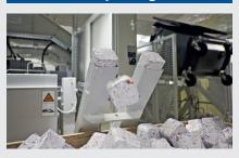
As an option, the Hunkeler Document Destruction System HDDS 30 can be supplemented with a briquetting press. The press compacts the particles into dense briquetts. Volume is reduced by a ratio of 1:12, with a density of 1 kilo per cubic decimeter. Dust, which is produced during the shredding process is also included in these briquettes, resulting in a cleaner ambient air.
