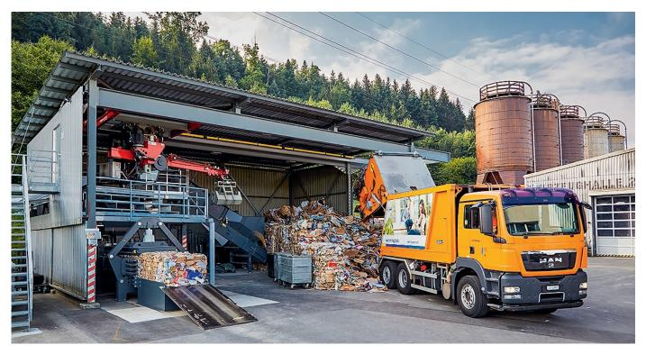
Annually, the Waste and Recycling Centre Ibach compacts about 2,000 tons of cardboard to bales. The resultant material is then recycled for the production of corrugated cardboard.
