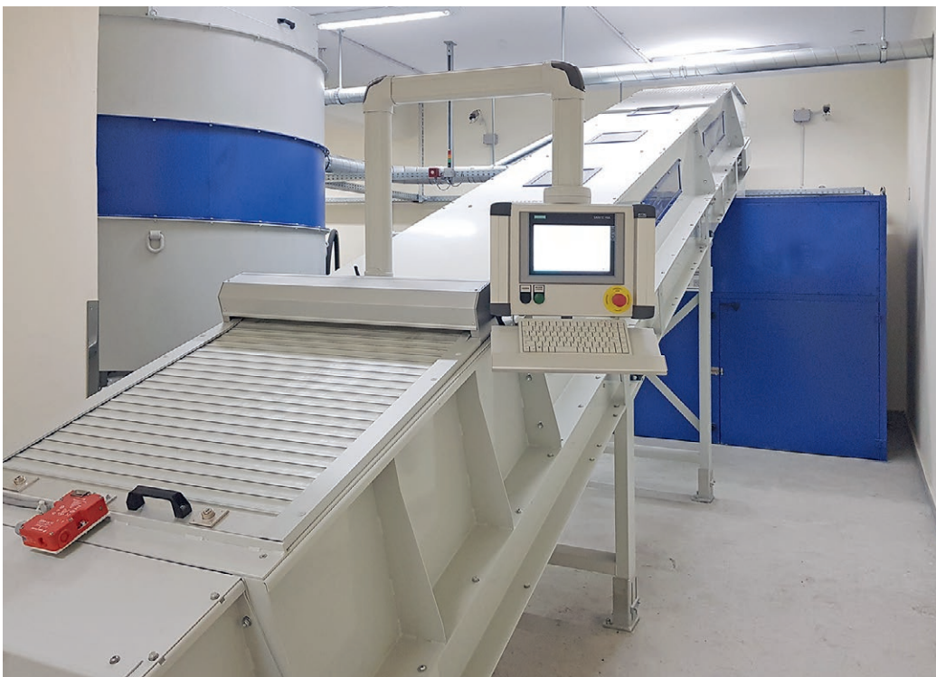
The disintegration systems by Hunkeler Systeme AG are based on a maximum destroying capacity of 300 kilograms per hour.
