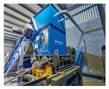
In the four-shaft shredder, a robust cutting unit processes paper, carton as well as pieces of metal.
