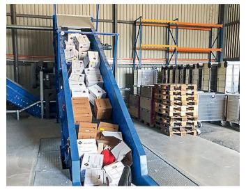
Loose sheets, cardboard boxes and complete binders are reduced in the system to particles according to security level P4.
