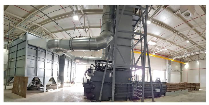
To ensure that the great quantity of cardboard waste is reliably disposed of in 24/7 operation, Hunkeler Systeme AG installed two high performance baling presses from the series VK 4212. The cardboard waste is transported to the presses via paper cutters.
