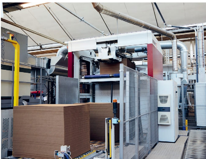
The plant processes the material on six flatbed die cutters and five inliner rotary die cutters.
