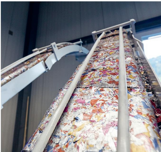
After crushing, a press processes the aluminium particles to briquettes with a density of 1.8 to 2 kilograms per cubic decimetre.
