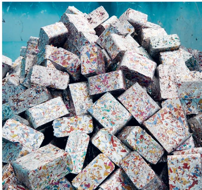
Thanks to the briquetting press, Leuthold Mechanik AG achieves a volume reduction of around fifty times that of non-compacted material.
