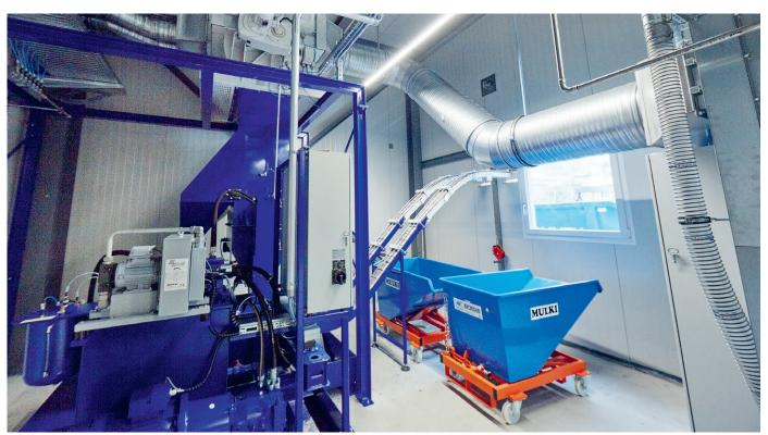
Leuthold Mechanik AG currently has 40 machines connected to four extraction and compaction systems from Hunkeler Systeme AG. The production technology is soon to be expanded.
