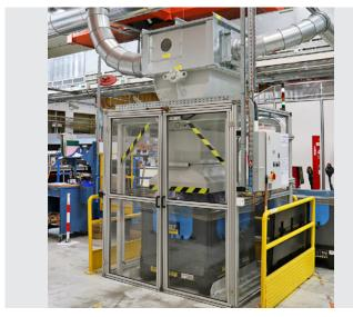
The margin strips are separated in a rotary cutter from the transport air and automatically compressed in a container.
