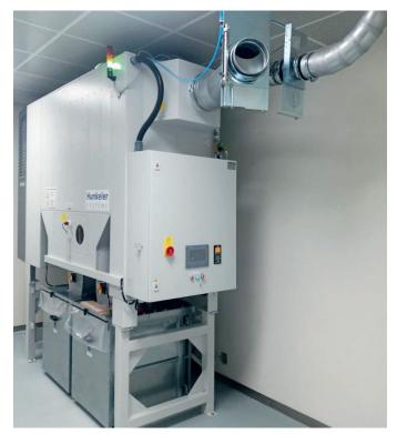
The HKU 4510 is prepared for connection (see above in the photo) to an offline shredder.
