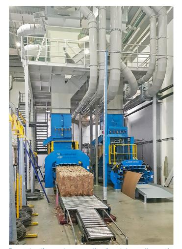
Two extraction and compaction lines take on the waste from a dedicated corrugated cardboard production line. They also serve simultaneously as a back-up for each other.
