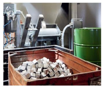
Per recycling circuit up to 99.5 percent of the original material quantity can be re-used after the shavings have been compacted to briquettes.
