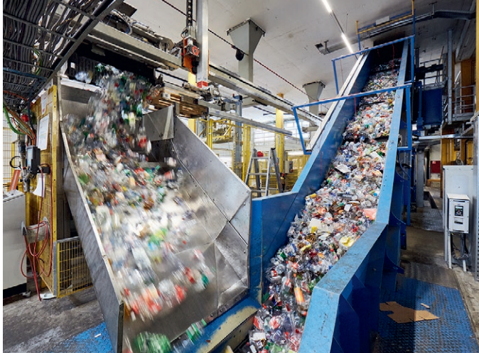
A robot empties the containers into a feed hopper, and the waste reaches the baler via an ascending belt.
