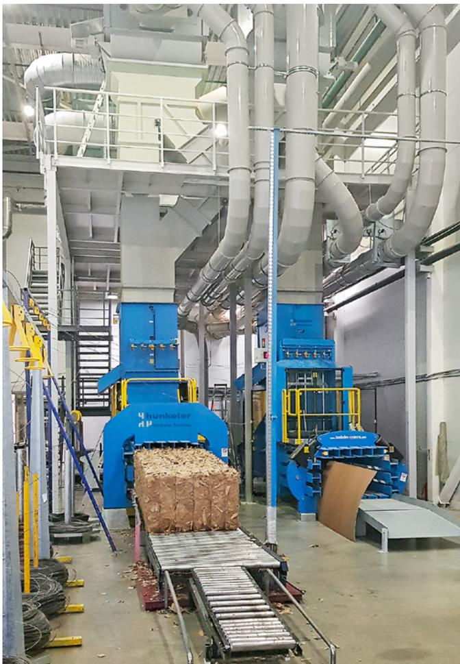
Two extraction and compaction lines take on the waste from a dedicated corrugated cardboard production line. They also serve simultaneously as a back-up for each other.
