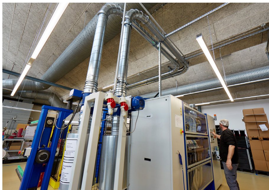
At a web speed of 600 metres per minute, the plastic strips are shredded in the cutting unit and disposed of via pipelines.
