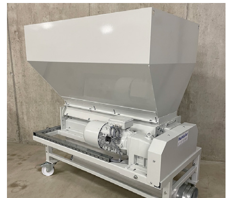
The SAZ stripping waste shredder shreds the waste at the centre break-out station.
