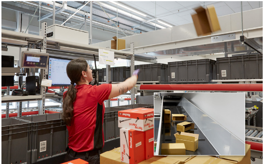
A conveyor belt (small picture) transports the emptied cardboard boxes to the outside area, where the boxes are compacted in a press container.
