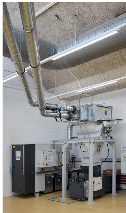
A constant suction performance and ring ionisers ensure a smooth and stable process when disposing of the plastic material.
