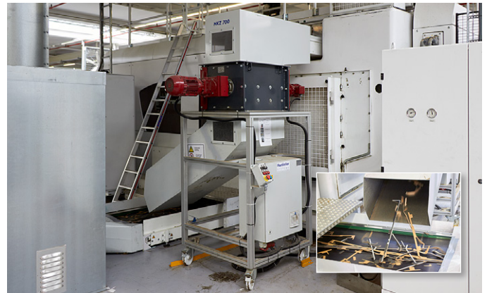
The HKZ-700 shredder also shreds larger gripper margins with widths of up to 150 millimetres without any problems.
