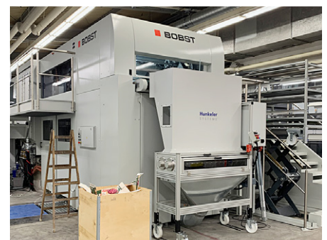
The SZM shredding module was developed for energy-efficient disposal of the waste grids and gripper margin.
